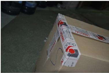
B. After application, tape should be smoothed with a dispenser or hand in a way its whole surface sticks to a box.
